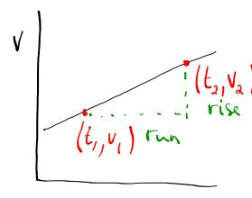
$$\text{slope} = \frac{\text{rise}}{\text{run}}$$
